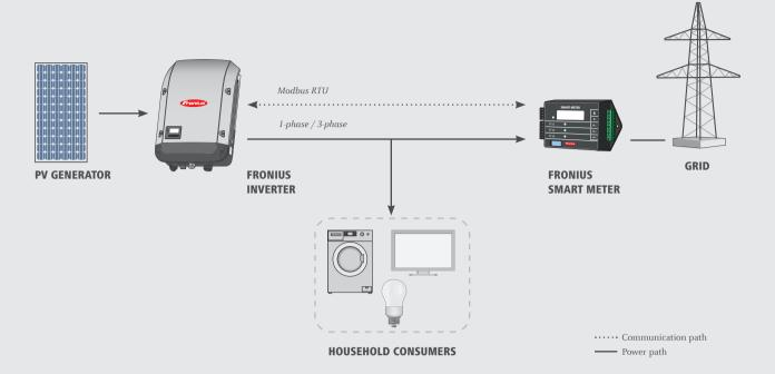
/ The Fronius Smart Meter is compatible with all inverters with an RS485 interface (Modbus RTU). The Fronius Smart Meter works in conjunction with the Fronius Datamanager 2.0 for the Fronius IG Plus inverters. The Fronius Smart Meter can be retrofitted at any time together with the Fronius Datamanager 2.0 in inverters that have already been installed.
